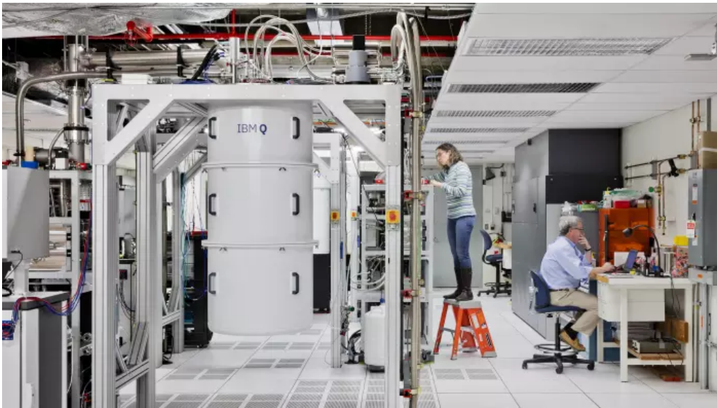
The IBM Q quantum computer, which can be accessed by companies via IBM's cloud operation © Connie Zhou/IBM
