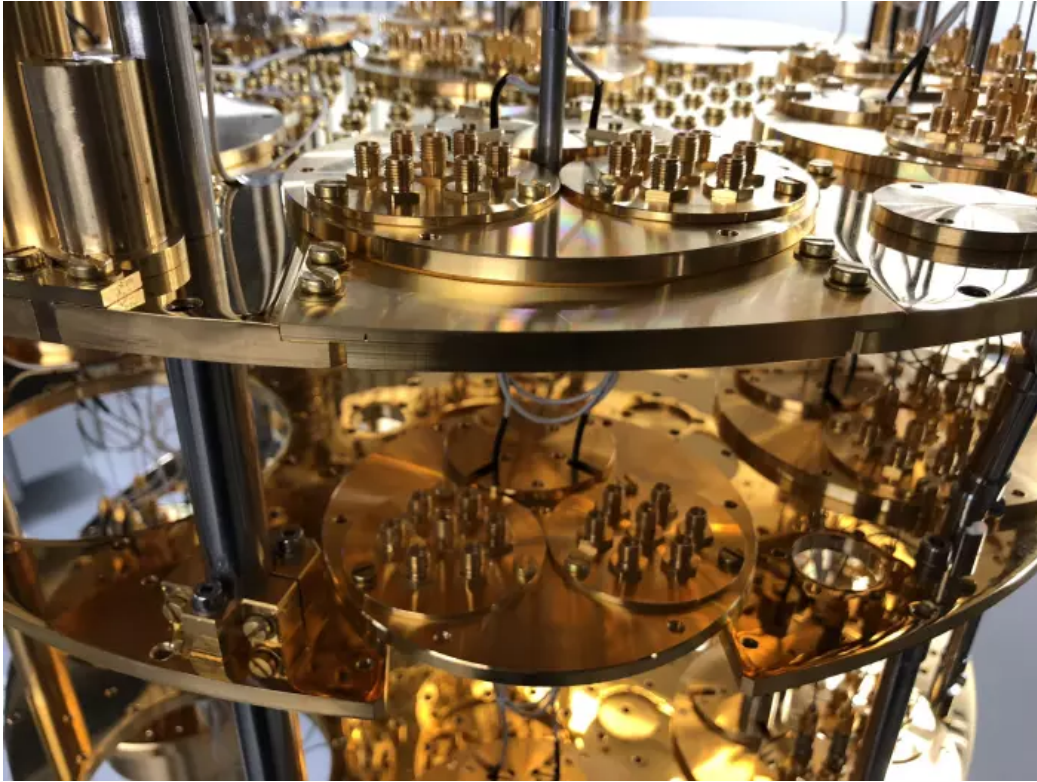
Inside a Bluefors quantum chip cooler at University College London
