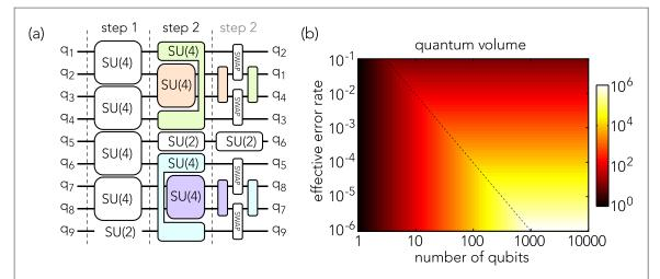
**Figure 2.** (a) Example quantum circuit with two circuit steps. Step 2 requires different connectivity and would lead to an increased gate count on quantum hardware with only nearest neighbor interactions. This is illustrated to the right of step 2. (b) Quantum volume as a function of the effective error rate  $\epsilon_{\text{eff}}$  and the physical number of qubits N. For simplicity, we assume that for a given  $\epsilon_{\text{eff}} V_{\text{Q}}$  stays constant for d < N.
