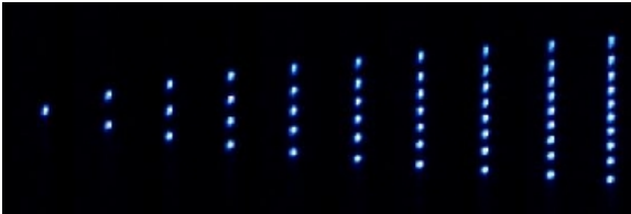
Sequential loading of Yb ions into a linear Paul trap. (physic.uni-siegen.de)
