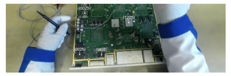
A technician repairs a circuit board using an augmented reality overlay at Ericsson's Tallinn factory. (Source: Ericsson)
