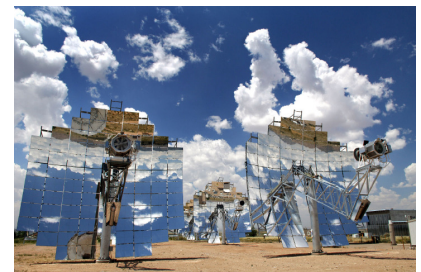
Figure 5. Stirling dish engine. These beautiful concentrators deliver a power per unit land area of 14 W/m 2 . Photo courtesy of Stirling Energy Systems. www.stirlingenergy.com
