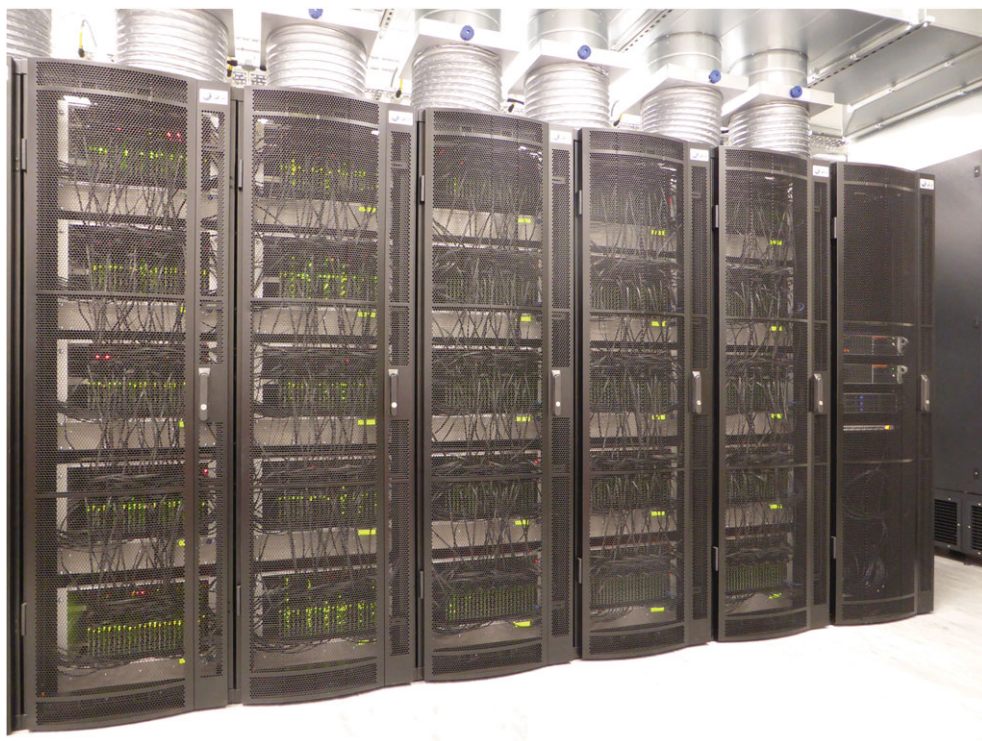
Figure 3. The SpiNNaker machine, delivered in 2016. The machine incorporates 28 800 SpiNNaker chips—half a million ARM processor cores in total—connected into a two-dimensional toroidal surface, contained in five 19" rack cabinets. The sixth cabinet contains the associated server systems. The total active silicon area in the machine amounts to 5 m 2 . (Online version in colour.)
