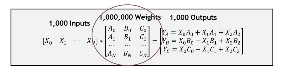
Weight data could need to be stored in *DRAM*, and it does not have the same amortization as the intermediate data
