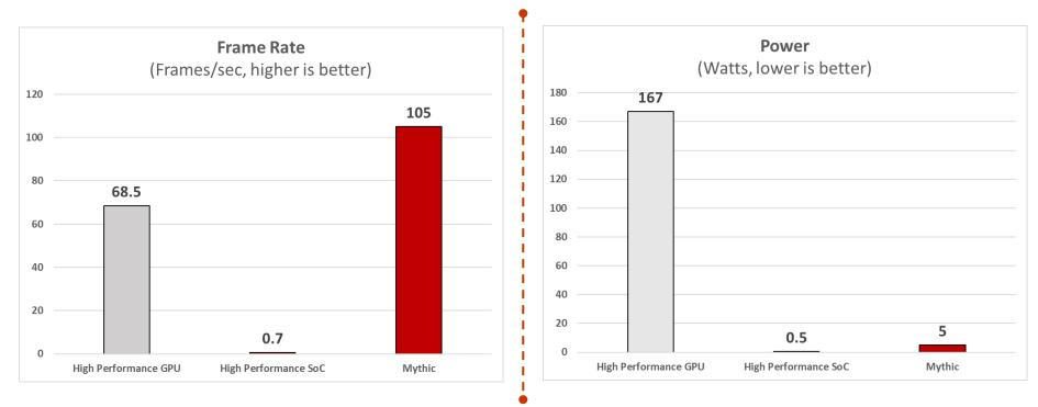
Running at 656x368 resolution. Mythic estimated, GPU/SoC measured
