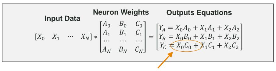
Key Operation: Multiply-Accumulate, or "MAC" Figure of Merit: How many picojoules to execute a MAC?
