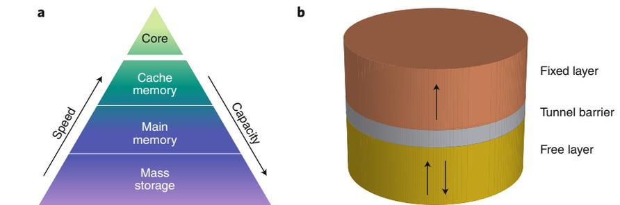
**Fig. 1 | Memory hierarchy and MTJ.** **a**, Schematic of memory hierarchy. The speed (capacity) is increased (decreased) for different levels of memories from the bottom to top. **b**, Schematic of an MTJ. The resistance state is determined by the relative magnetization direction (black arrows) between the fixed and the free layer. Magnetization of the free layer can be switched by driving a current across the junction.
