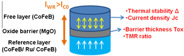
Fig. 1. Magnetic Tunnel Junction (MTJ) is mainly composed of three thin films: two ferromagnetic layers and one oxide barrier (e.g. CoFeB (1.2 nm)/MgO (0.85 nm) / CoFeB (2 nm)). It presents two resistance values ( R_P or R_{AP} ) depending on the relative magnetization of two ferromagnetic layers (Parallel or Anti-Parallel). The resistance difference is characterized by Tunnel Magnetoresistance Ratio (TMR) = (R_{AP} - R_P)/R_P [11]. Through Spin transfer torque mechanism, a low bidirectional current, I_{WR} higher than the threshold current I_{CO} can switch the MTJ between two states [1].
