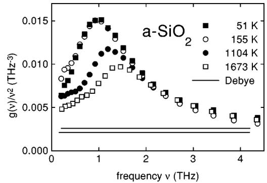
FIG. 2. Density of states of vitreous silica for four temperatures in the representation  $g(\nu)/\nu^2$  vs frequency. The solid lines represent the Debye density of states for the lowest (upper line) and highest (lower line) temperature.
